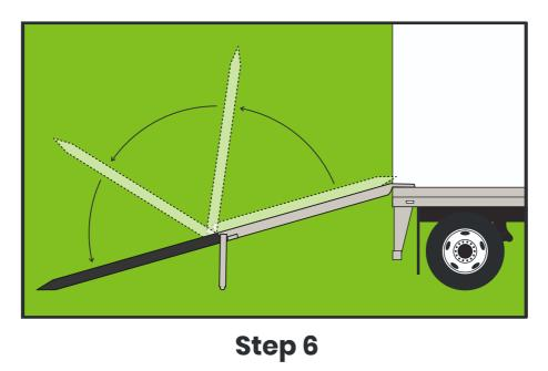
Unfold ramp, resting it on ground
