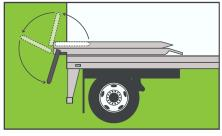
**Step 2**Unfold leg assembly until legs rest against stop blocks and lock into leg assembly
