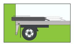
**Step 1**Slide ramp towards you until leg assembly is clear of the trailer
