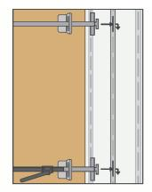
**Step 2**Firmly press T-shaped load bar ends down into vertical trailer post slots
