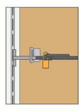
**Step 8**Place a lock in each handle to secure bulkhead
