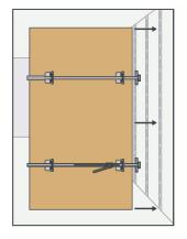
**Step 1**Align first bulkhead panel with vertical trailer post
