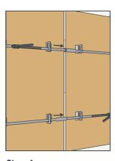
**Step 4**With handles open, slide load bars together until pinholes align
