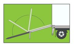
**Step 6**Unfold ramp, resting it on ground
