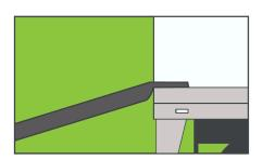
**Step 4**Ensure rail ends are touching end of trailer and entire apron is inside trailer
