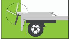
**Step 2**Unfold leg assembly until legs rest against stop blocks and lock into leg assembly
