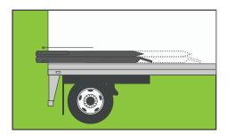
**Step 1**Slide ramp toward you until leg assembly is clear of the trailer
