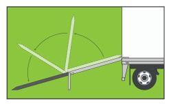
**Step 6**Unfold ramp, resting it on ground
