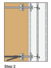
Firmly press T-shaped load bar ends down into vertical trailer post slots
