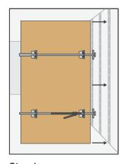
**Step 1**Align first bulkhead panel with vertical trailer post
