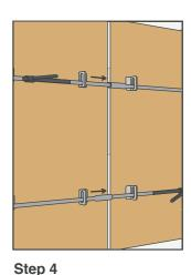
With handles open, slide load bars together until pinholes align
