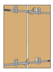
**Step 5**Insert locking pin through each load bar
